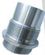
Adopter Mat: Tool Steel (HRC 47) Size: \varnothing 62 x 64 mm Precision: 0.02 mm
